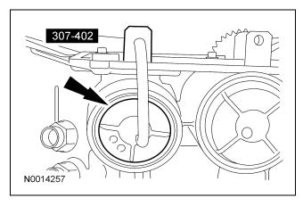
65. **NOTE:** If the overdrive band is reused, it must be installed in the same position as when removed.
